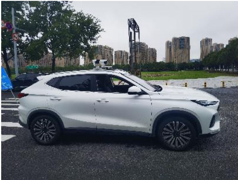
Fig. 1: The modified experimental vehicle used in our illegal behaviors detection system
